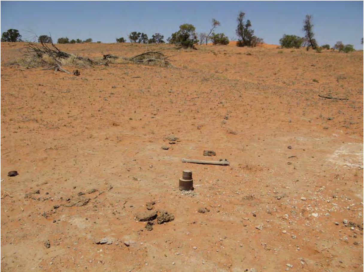
Figure 1. Yalkalpo 2 collar – note cement plug
